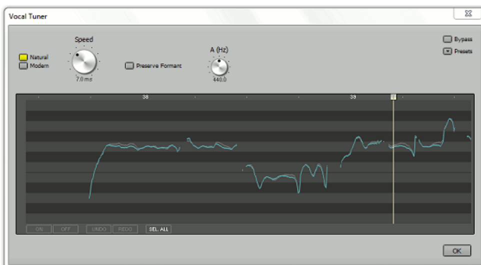
Vocal Tuner window: gray curve is input, blue curve is output pitch
